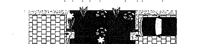
Permeable Pavement w/Micro-Bioretentation - Plan View NOT TO SCALE
