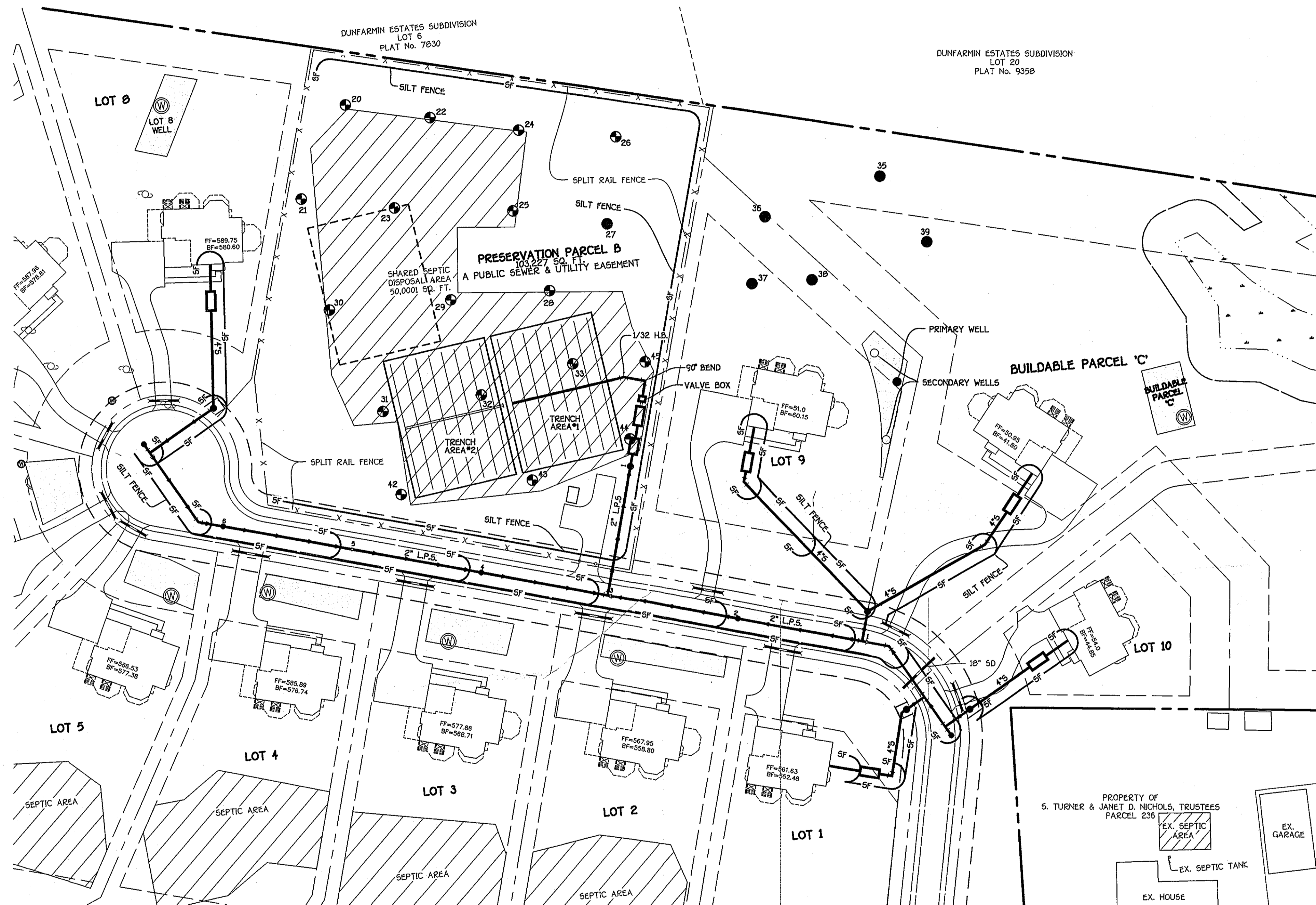
EROSION & SEDIMENT CONTROL PLAN SCALE: 1"=50'
