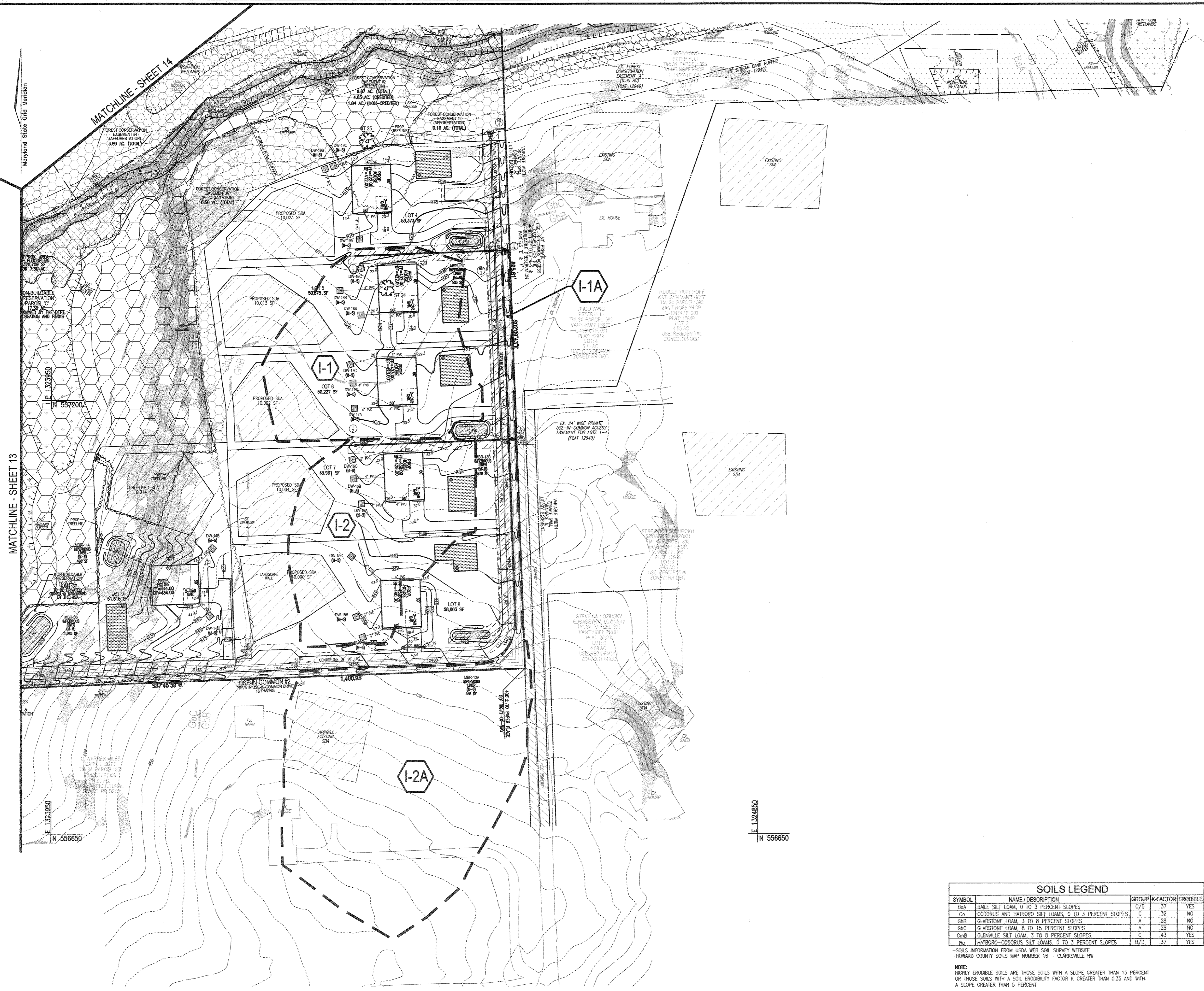
SD DRAINAGE AREA MAP SCALE: 1"=60'
