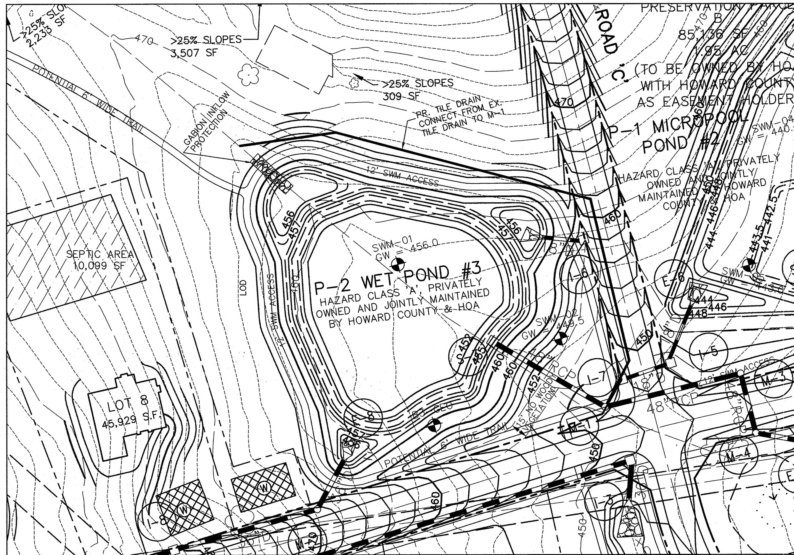
STORMWATER MANAGEMENT POND #3 SCALE: 1"=50'
