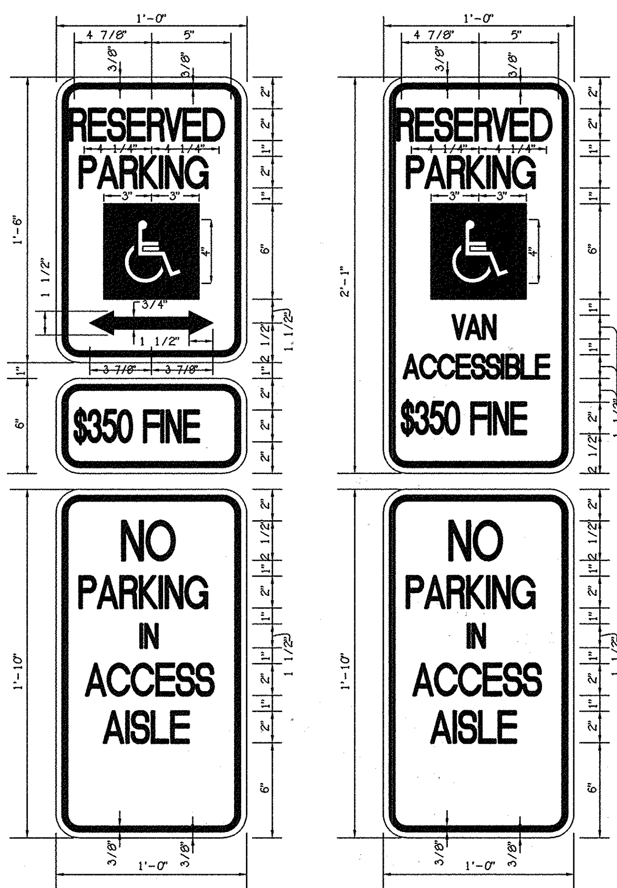
8 HANDICAP PARKING SIGN DETAIL NOT TO SCALE
