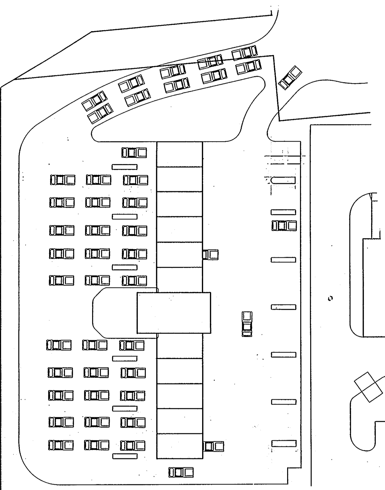
OFF STREET PARKING RESERVOIR DETAIL NO SCALE
