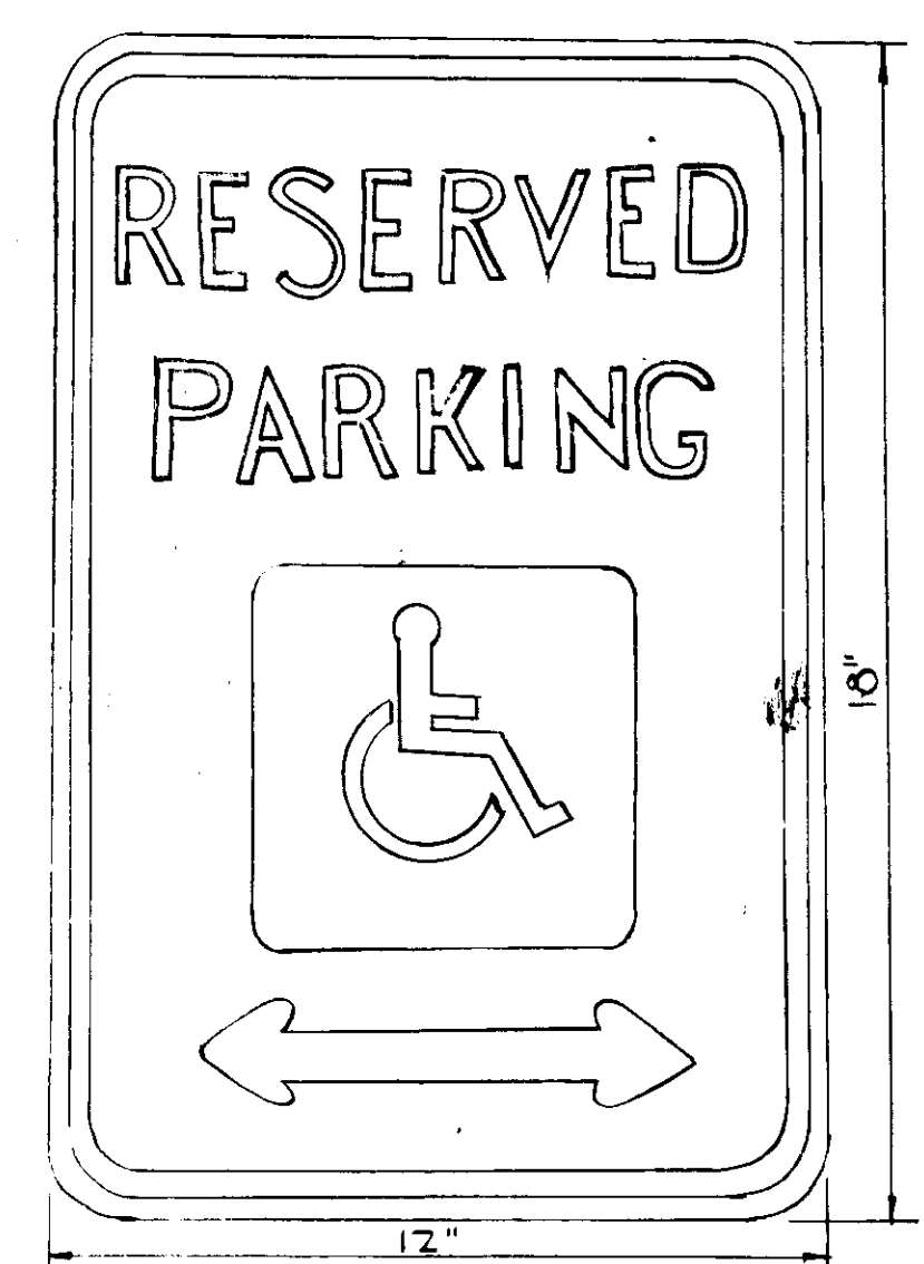
HANDICAPPED PARKING SIGN DETAIL
