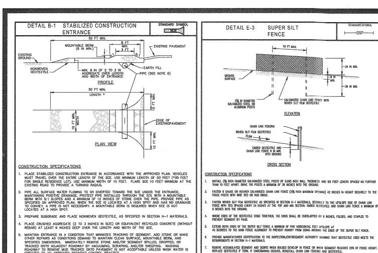
MARYLAND STANDARDS AND SPECIFICATIONS FOR SOIL EROSION AND SEDIMENT CONTROL
