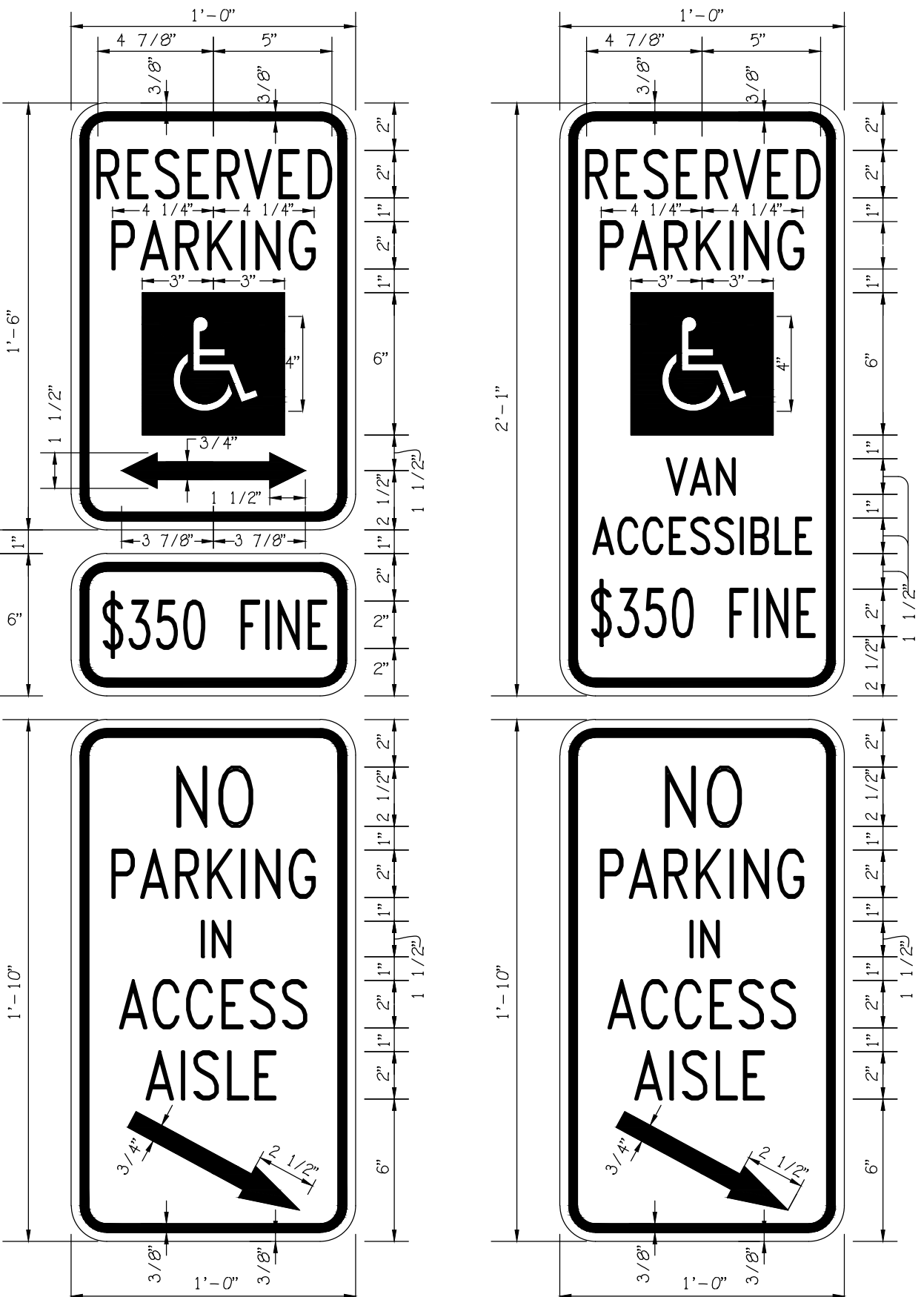
6 9 HANDICAP PARKING SIGN DETAIL NOT TO SCALE
