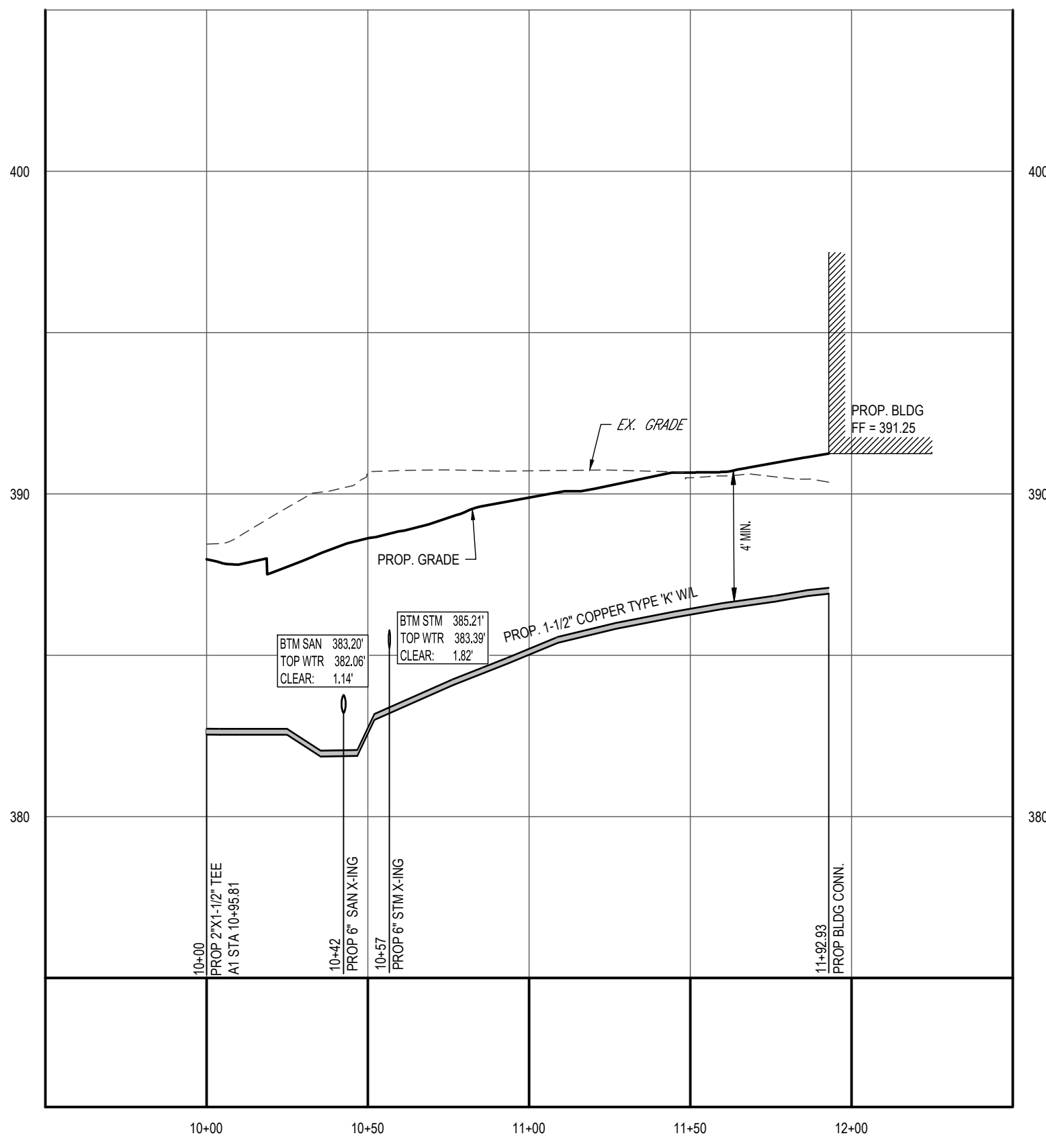
PROPOSED WATERLINE PROFILE - A2 SCALE: 1"= 40' HORIZONTAL 1"= 4' VERTICAL
