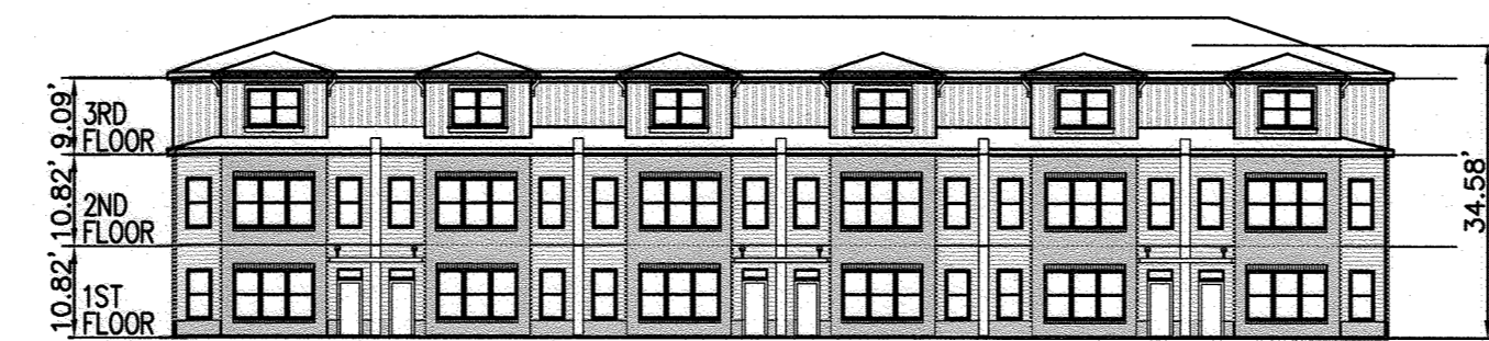
BUILDING 'B' - FRONT ELEVATION FIBER CEMENT CLAPBOARD, VINYL BOARD AND BATTON AND BRICK VENEER SIDING
