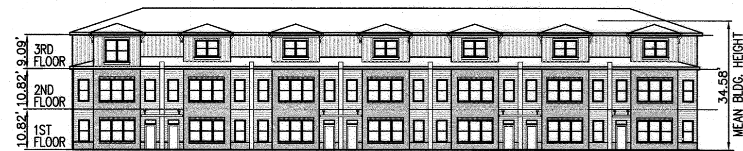
BUILDING 'C' - FRONT ELEVATION FIBER CEMENT CLAPBOARD, VINYL BOARD AND BATTON AND BRICK VENEER SIDING
