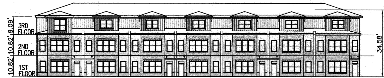
BUILDING 'A' - FRONT ELEVATION FIBER CEMENT CLAPBOARD, VINYL BOARD AND BATTON AND BRICK VENEER SIDING
