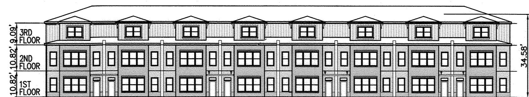
BUILDING 'D' - FRONT ELEVATION FIBER CEMENT CLAPBOARD, VINYL BOARD AND BATTON AND BRICK VENEER SIDING
