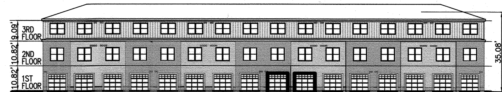
BUILDING 'D' - REAR ELEVATION FIBER CEMENT CLAPBOARD, VINYL BOARD AND BATTON AND BRICK VENEER SIDING
