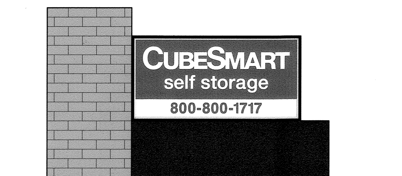
2 MONUMENT SIGN - FRONT ELEVATION SCALE: 3/4" = 1'-0"
