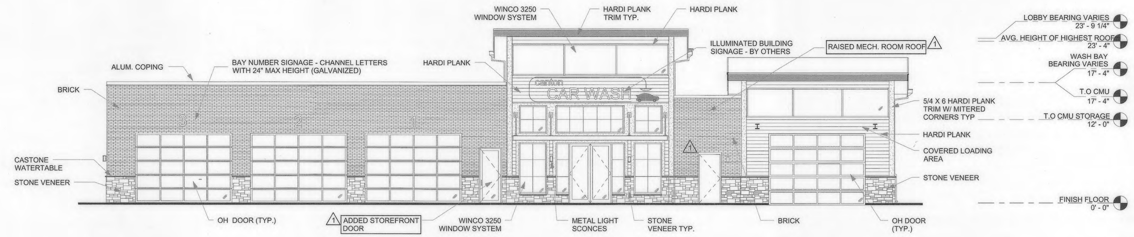
1 SOUTH ELEVATION 1/8" = 1'-0" NOTE: 1. SETBACK TO BE INCREASED BY 4'-0" PER FD-35-A AS AVERAGE HEIGHT OF HIGHEST ROOF (24'-0") IS HIGHER THAN 25'-0"
