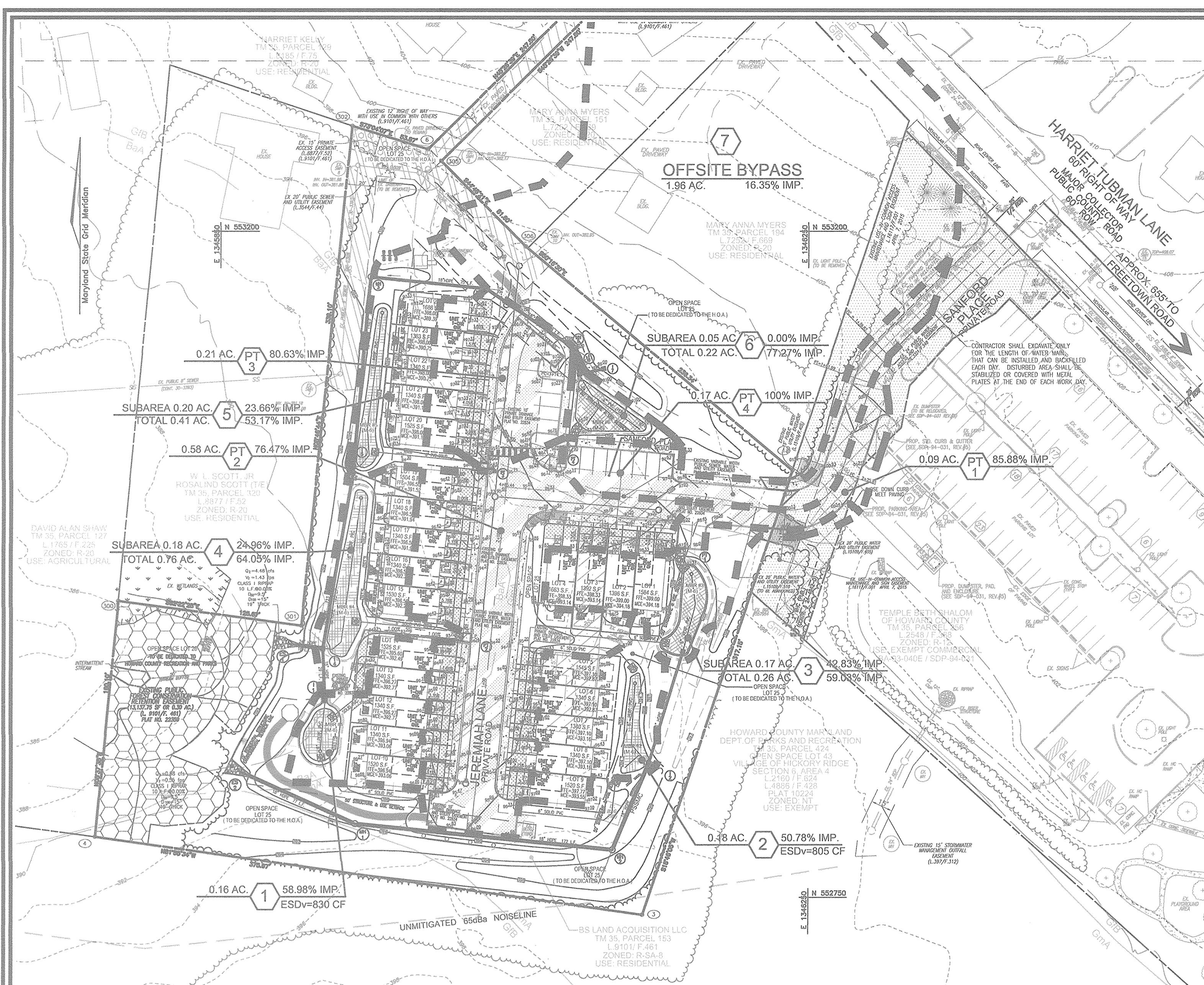
STORM DRAIN DRAINAGE AREA MAP SCALE: 1"=50'
