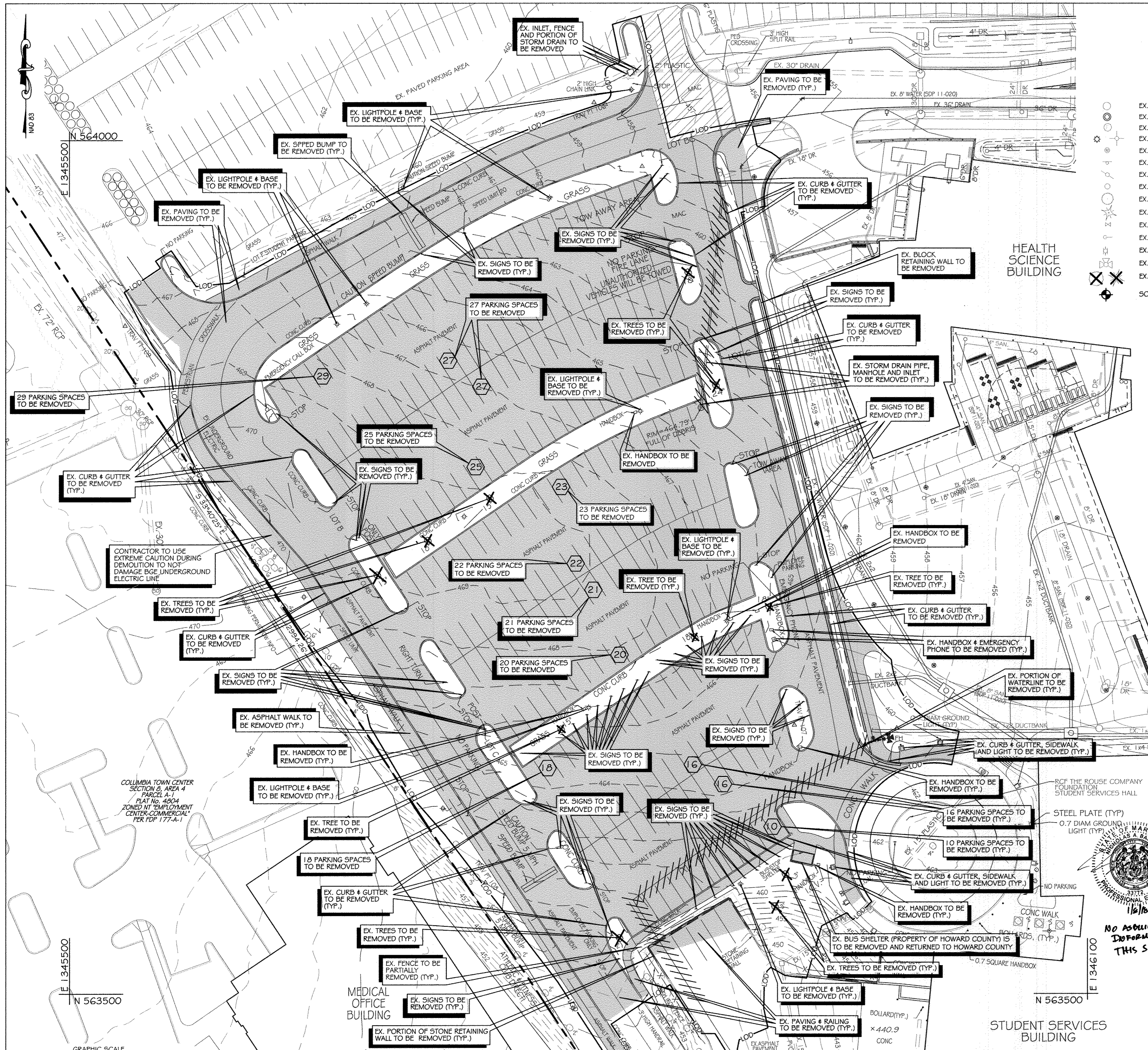
MATCHLINE SEE THIS SHEET FOR CONTINUATION EXISTING CONDITIONS / DEMOLITION PLAN SCALE: 1" = 30'
