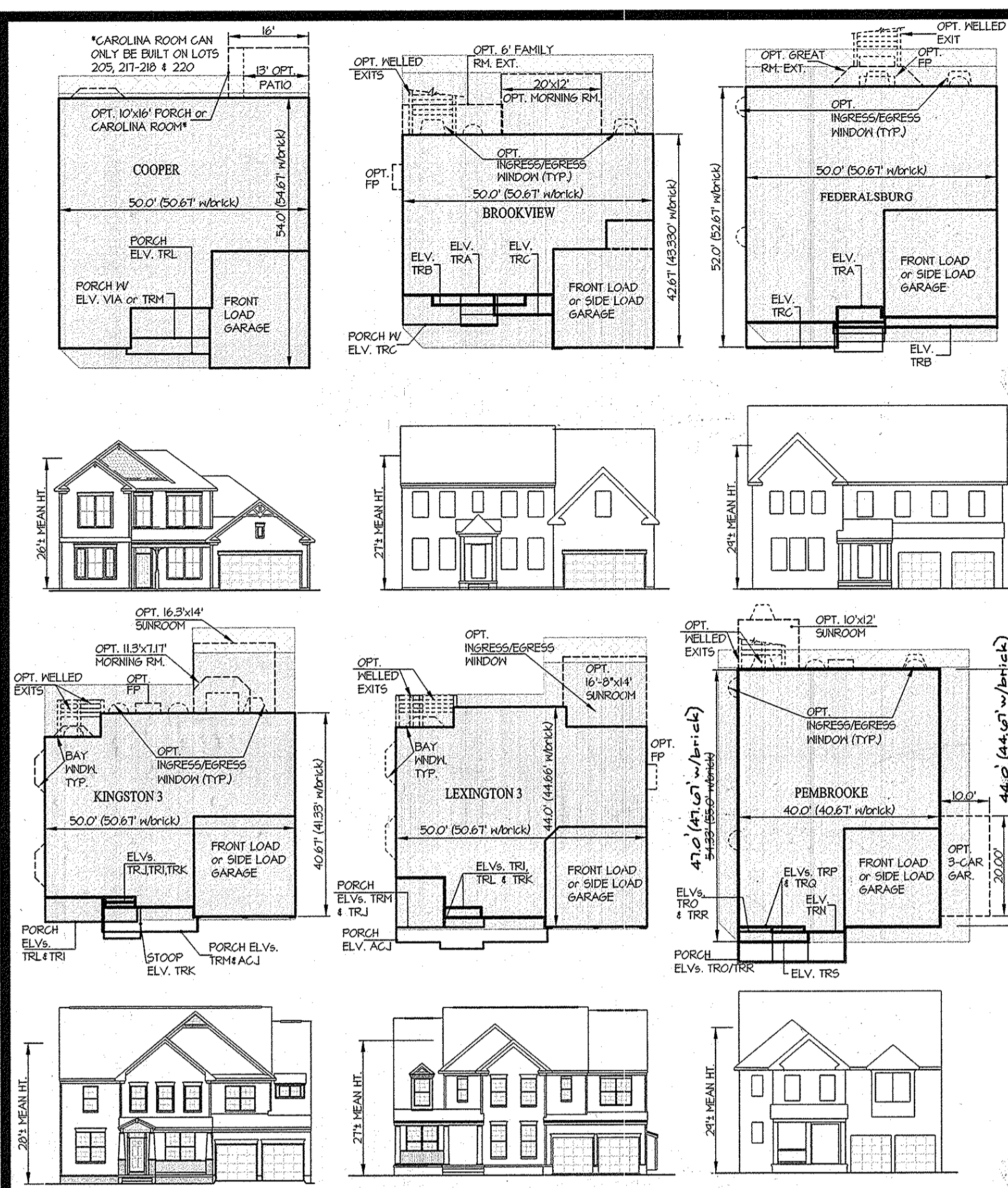
TYPICAL HOUSE FOOTPRINTS and ELEVATIONS (STANDARD (STD) ORIENTATION SHOWN) SCALE: 1" = 20'
