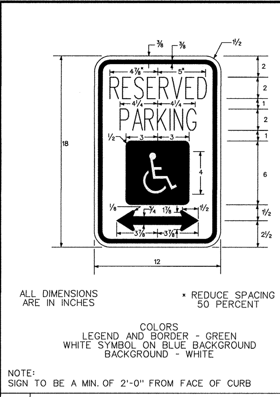
1 Not To Scale Detail Handicap Parking Signs
