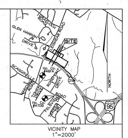
THE BEARINGS, COORDINATES AND ELEVATIONS USED IN THIS SURVEY ARE BASED ON HOWARD COUNTY CONTROL POINT NOS. 46FA N535140.866 E1346962.69 ELEV.403.65 N534316.917 E1348131.25 ELEV.398.56 47DB
