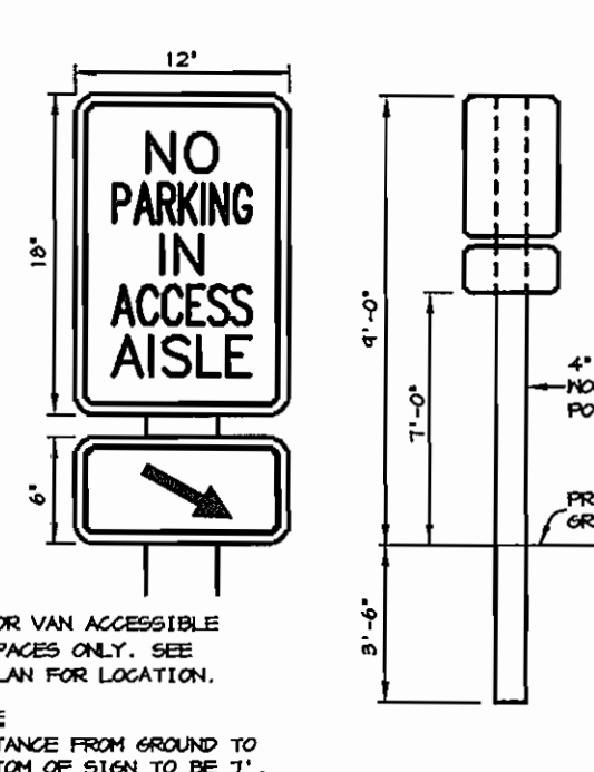
ACCESS AISLE SIGN NO SCALE
