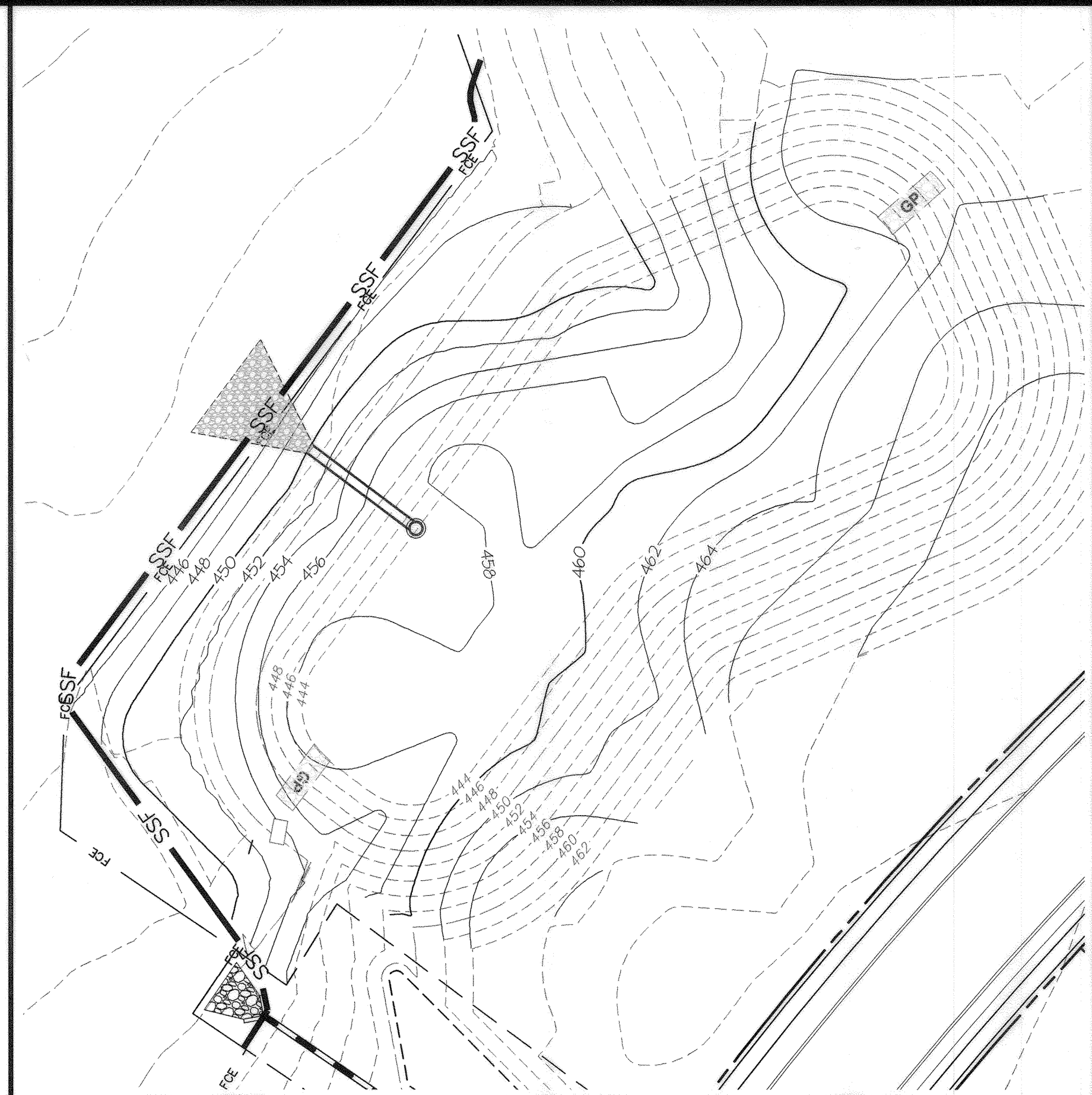
BACKFILL DETAIL - SEDIMENT BASIN 3 SCALE: 1"=30'
