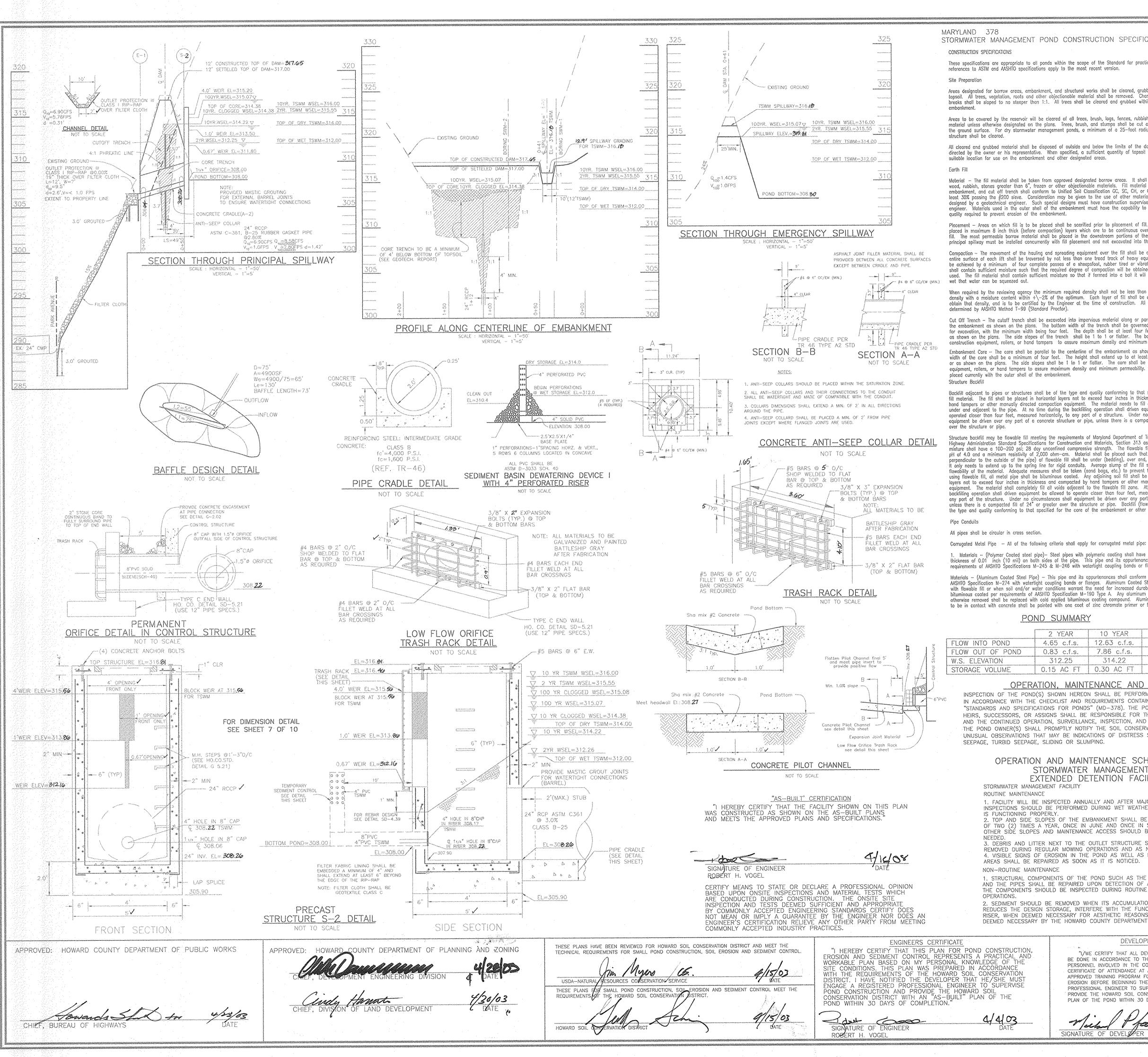
STORMWATER MANAGEMENT POND CONSTRUCTION SPECIFICATIONS CONSTRUCTION SPECIFICATIONS
