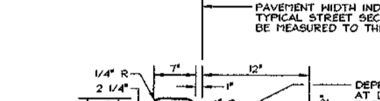
STANDARD COMBINATION CURB AND GUTTER HOWARD COUNTY STANDARD R-3.01 NOT TO SCALE
