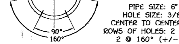
SCH40 PVC PERFORATED UNDERDRAIN PIPE DETAIL FOR HORIZONTAL DRAIN PIPE NO SCALE
