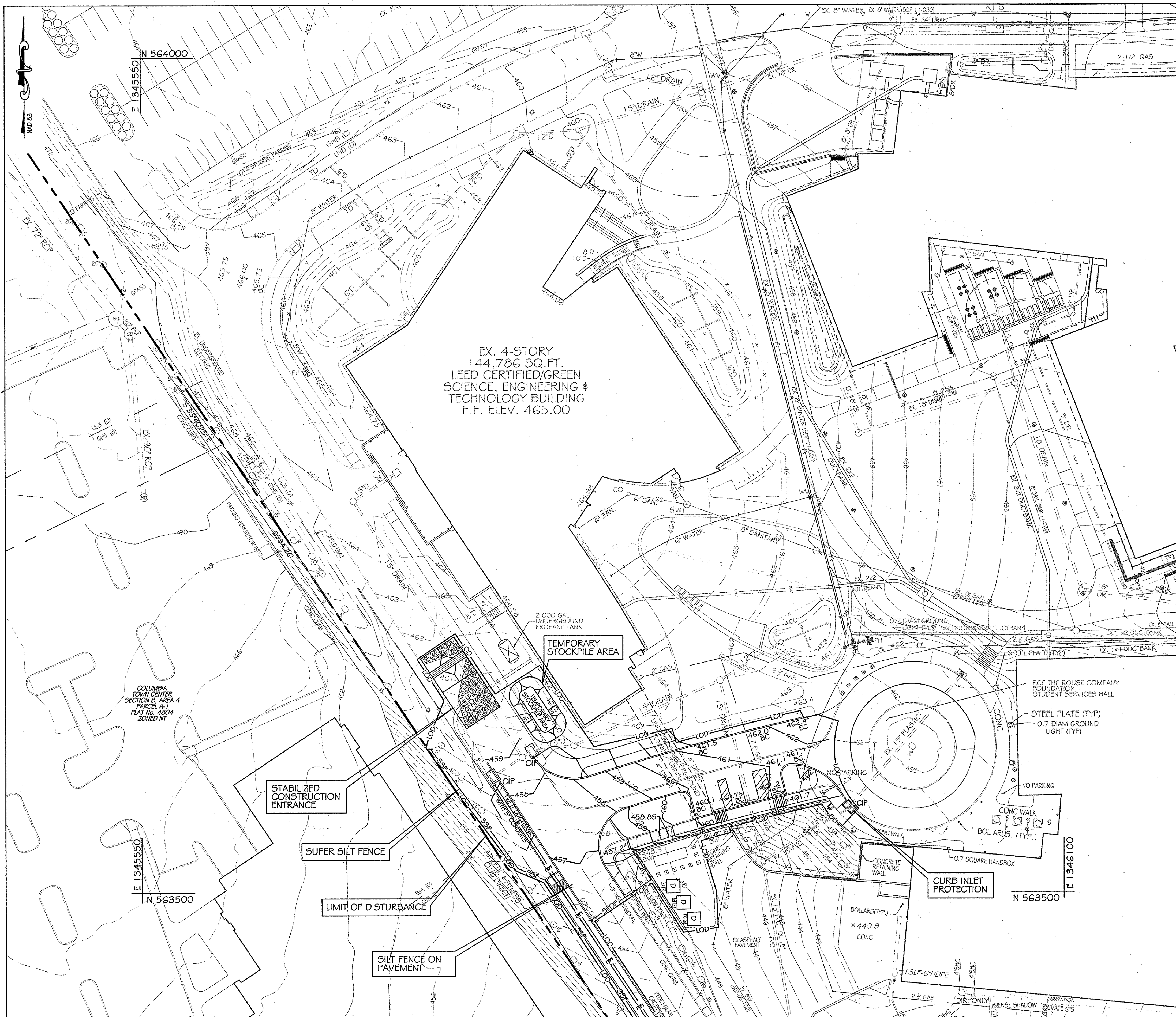
EROSION AND SEDIMENT CONTROL PLAN PHASE 4 SCALE: 1" = 30'
